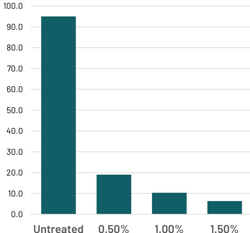
A customer's mortar mix treated with GC10-70LD. Dust value tested on Palas® DustView Analyzer
